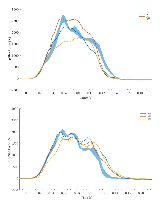
Figure 1 Time history of the upper shoulder seat belt force. Top: first series of PMHS tests (solid lines) and corridor response of corresponding THOR tests (shaded blue area). Bottom: second series of PMHS tests (solid lines) and corridor response of corresponding THOR tests (shaded blue area).
