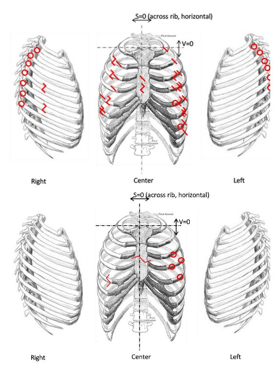
Figure 2 Approximate location of the rib and sternal fractures observed in the post-test PMHS examination. First PMHS series above (PMHS1: angled line; PMHS2: straight line; PMHS3: circle). Second PMHS series below (PMHS4: angled line; PMHS5: straight line; PMHS6: circle
